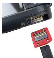
Charging and file transfer through the waterproof USB port
