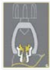
Picture C: Yoke regulator disconnected > regulator closed
